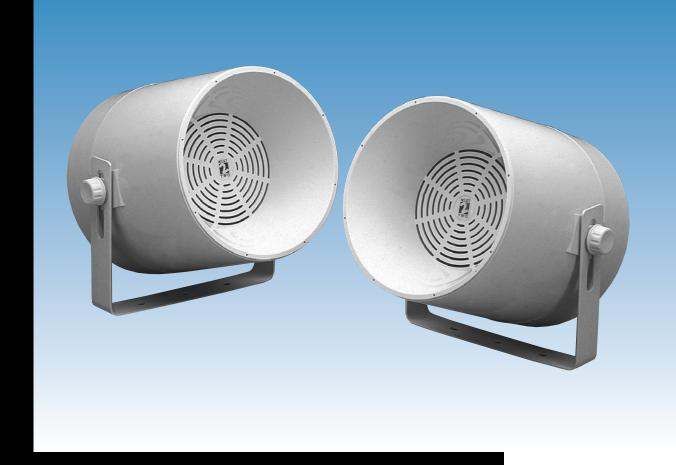
A 20 Watt cream outdoor music sound projector manufactured in ABS plastic with a metal bracket. This projector is completely weatherproof (IP54) and offers both clear speech and excellent quality background music reproduction. This unit is supplied complete with 100 volt line transformer but can also be used as an 8 ohm low impedance unit.
