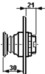
Mushroom-head pushbutton actuator "EMERGENCY STOP"
