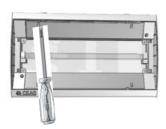
single sided luminaire 28011: lift top cover by loosing the 4 fixing screws.
