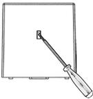
Press the snap hooks together by help of a suitable screw driver and pull the cover of the luminaire down.
