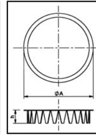
Rondelle de continuité Lead sheath earthing washer
